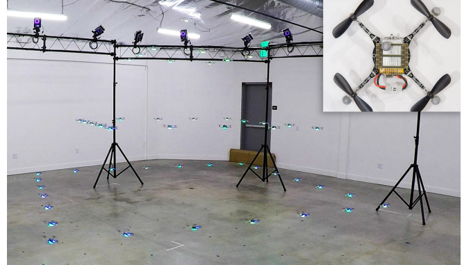
Fig. 1. Forty-nine Crazyflies flying in a four-layer rotating pyramid formation. The bottom layer is 3 \times 3 m with 0.5 m spacing between vehicles. A video of this flight is available at https://youtu.be/ezTayb76x9U . Inset: Crazyflie 2.0 quadcopter with motion capture markers.
