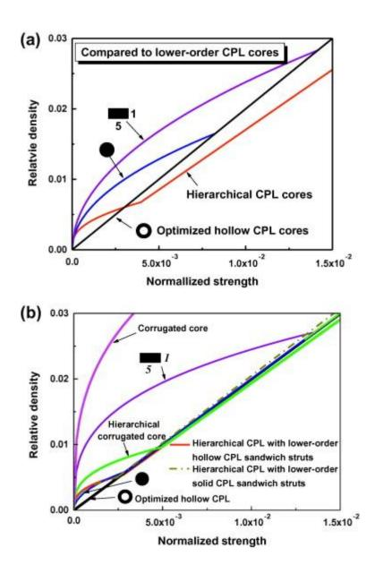
Fig. 10. Structural efficiencies of hierarchical CPL cores (a) compared to lower-order CPL cores with different trusses as shown with insets (solid/hollow round or rectangular trusses) and (b) comparison after homogenization of component materials.
