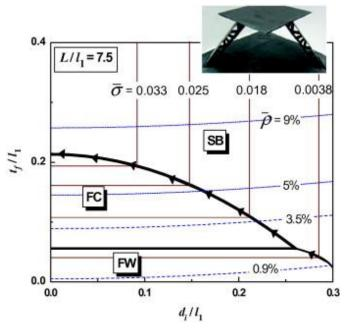
*Fig. 11.* Collapse mechanism maps of hierarchical corrugated core with hollow CPL sandwich struts of  $L/l_1 = 7.5$ .
