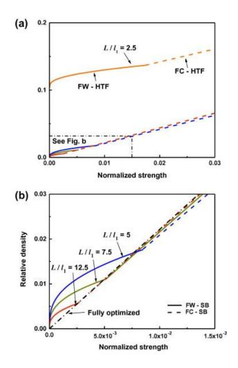
Fig. 9. (a) Normalized strength for the hierarchical CPL cores with specific L/l<sub>1</sub> and (b) the enlarged drawing of (a).
