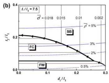
**Fig. 8.** Collapse mechanism maps with (a)  $L/l_1 = 2.5$  and (b)  $L/l_1 = 7.5$ . Note that the arrows in (b) designate the path of optimum designs with increasing relative density  $\bar{P}'$ .
