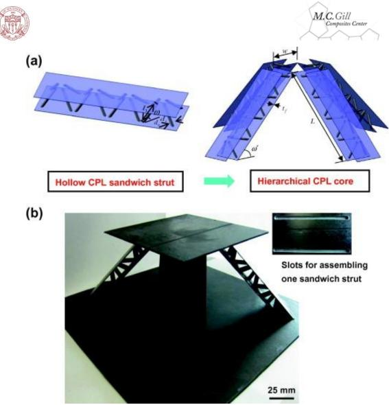
Fig. 2. (a) Illustration for building hierarchical periodic structures: from composite pyramidal lattice (CPL) core sandwich to hierarchical CPL core and (b) prototypical hierarchical CPL core sandwich structure.
