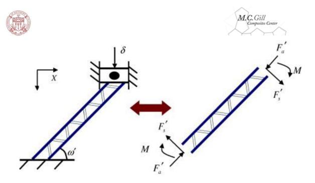
Fig. 3. Analysis for one sandwich strut of hierarchical CPL cores in out-of-plane compression.
