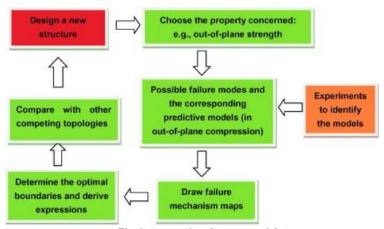
Fig. 1. A protocol guiding structural design.
