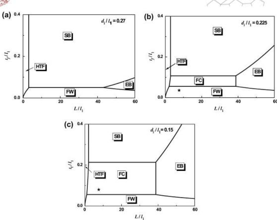
Fig. 5. Failure mechanism maps for the hierarchical CPL sandwich structure in out-of-plane compression constructed as a function of face sheet parameters  $t_f/l_1$  and  $L/l_1$  for: (a)  $d_f/l_1 = 0.27$ , (b)  $d_f/l_1 = 0.225$ , and (c) $d_f/l_1 = 0.15$ . (SB = shear buckling; FW = face sheet wrinkling; FD = face sheet delamination; EB = Euler buckling; HTF = hollow truss fracture).
