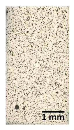
Figure 1. Digital image correlation pattern of cuboidal sample.
