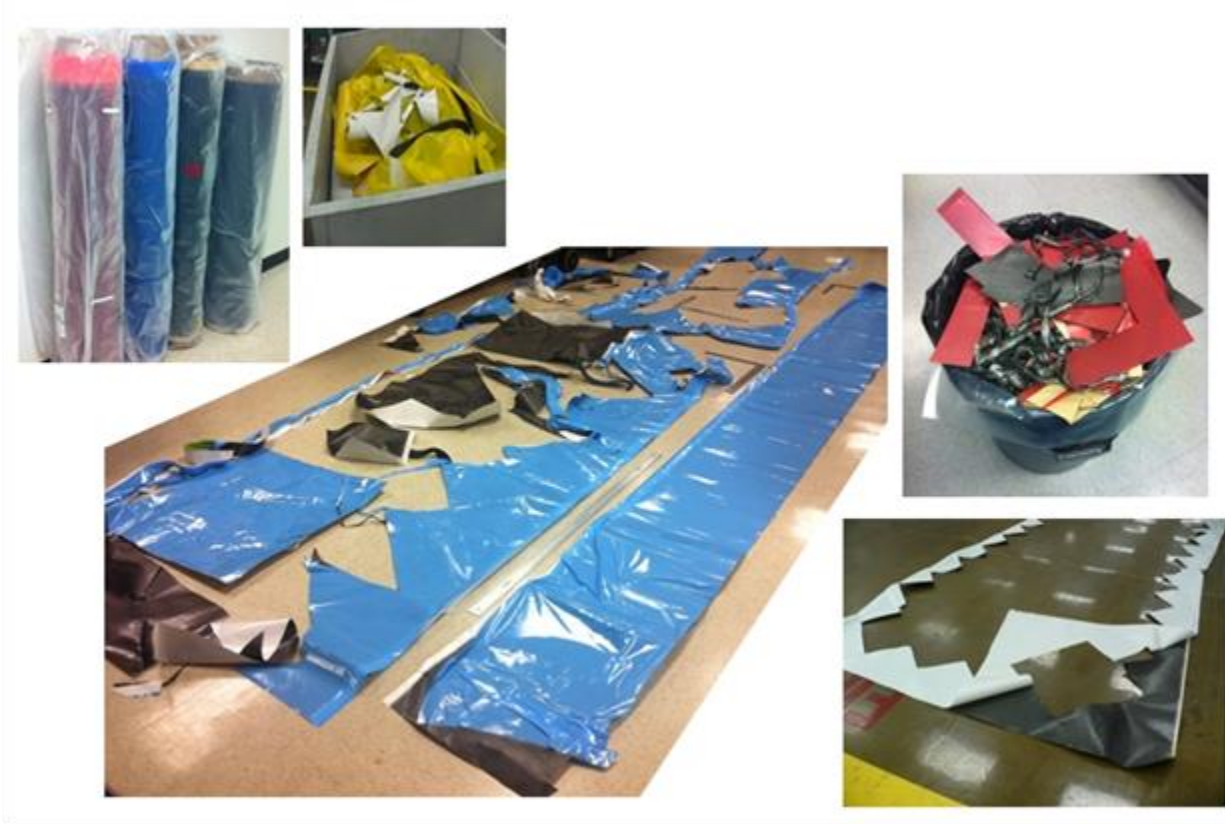
Figure 1: Exemplary uncured scrap prepreg – ply cutter scrap and out-timed rolls
