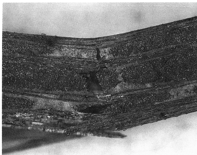
Fig. 6. Failure occurred at the loading points during creep-rupture experiment.
