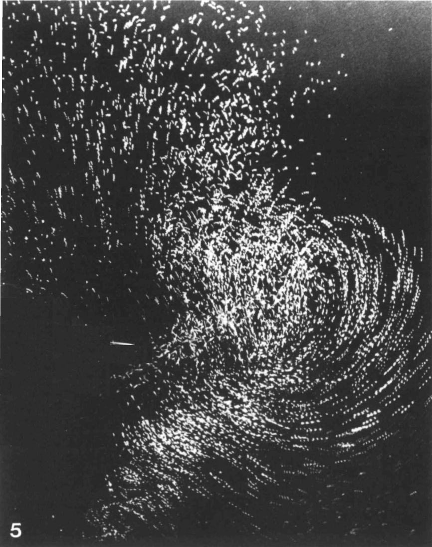
Fig. 5. The location of the downstroke trailing vortex is marked by axial flow along the core. Careful inspection of this photograph shows the connection between upstroke and downstroke trailing vortices. A starting vortex connecting the two sides of the wake would be here, if present, but was observed in none of the wake photographs. Mean flash interval was 16 ms.
