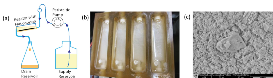
Figure S1. Growth and characterization of mature P. mirabilis crystalline biofilms on flat silicone substrates. (a) Schematic of the flow system. The silicone samples were submerged in (b) the modified drip flow reactor [1] and inoculated with a 4 hour culture of P. mirabilis . After allowing the bacteria to adhere for 1 hour, artificial urine with 1% tryptic soy broth was pumped at 0.5 \text{ mL min}^{-1} through the drip flow reactor and over the flat silicone samples. The reactor was maintained at 37^\circ\text{C} by mini-incubator. A mature crystalline biofilm grew over approximately 42 hours. (c) SEM of the resultant planar biofilm shows large crystals and microcrystal aggregates typical of mature P. mirabilis biofilms observed in catheters removed from infected patients. [2]
