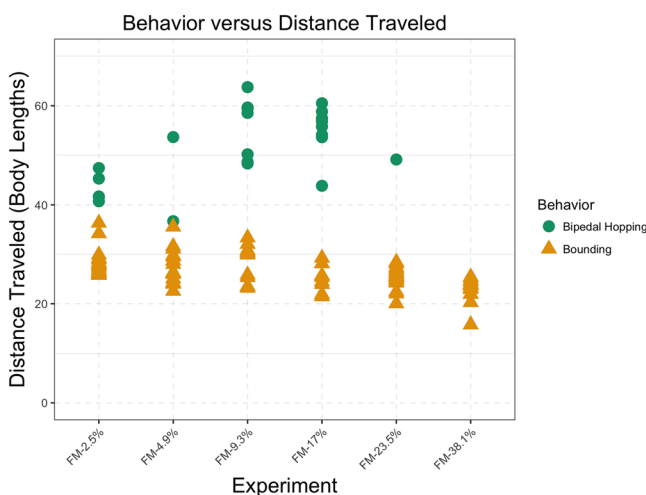
Figure 3. Behavior versus distance traveled for the farthest-traveling individual across the FM treatments. Each treatment comprises 20 replicate runs. Only replicates that produce bipedal hopping and bounding behaviors are included in this figure.
