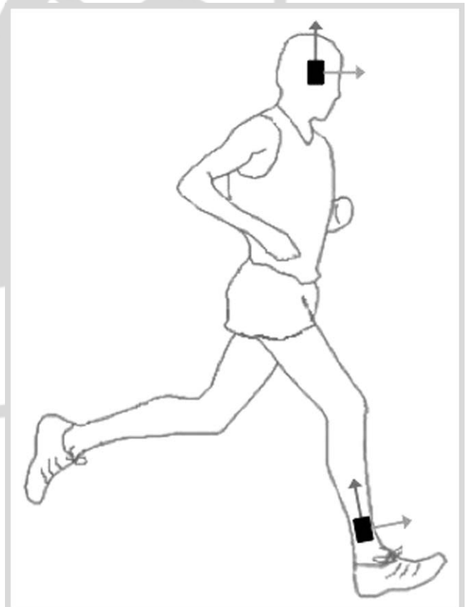
Fig. 1 Experimental set-up showing accelerometer placement and orientation of accelerometer axes.
