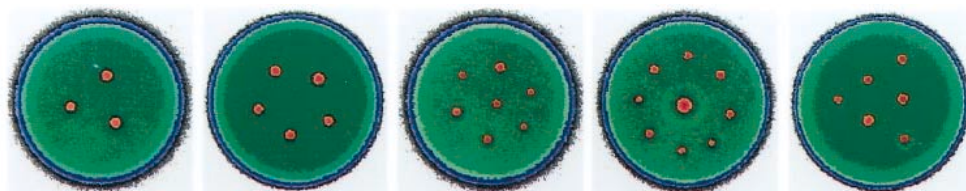
Fig. 1.15 Lattices with N = 3, 5, 7, 9, 6 formed in a magnetically confined nonneutral plasma, from Fine et al. (1995) (reprinted with permission from APS), which mimic some of the patterns produced in Campbell and Ziff (1978, 1979) as well as those shown in Figures 1.2 and 1.13. The vortices are magnetically confined pure electron columns. Note that the case N = 9 appears to have a stronger vortex at the center, surrounded by 8 equal strength vortices around the circular perimeter.
