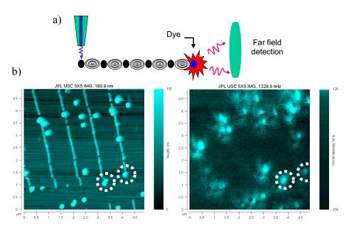
**Figure 8.** a) Schematic of the near-field excitation and far-field fluorescence detection scheme. b) topographic (left) and fluorescence intensity (right) plot of a 5x5 micron scan of fabricated plasmon waveguides with randomly deposited 100 nm dye beads. Two beads were pushed to the end of the nanoparticle arrays (white dotted circles) using the tip of an atomic force microscope.
