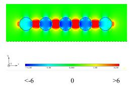
**Figure 4.** Distribution of the x-component of the electric field around an array of 5 Au nanoparticles in air excited at the collective plasmon resonance frequency by a propagating plane wave with the electric field polarized in the x-direction. The field enhancement inside and between the particles is due to dipolar near-field interactions.
