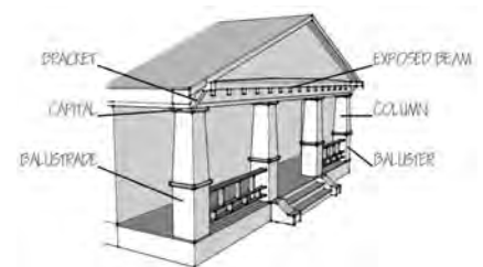
The components of a Craftsman style porch are shown
