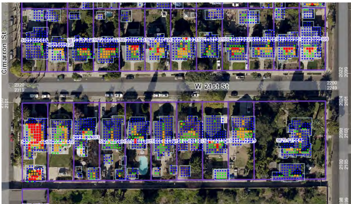
Fig 4.10: The solar map of a portion of the Western Heights HPOZ; the red color shows the best access to solar resources while the orange color shows good access. Source: L.A. County Solar Map ( http://egisgdx.isd.lacounty.gov/solar/m/?viewer=solarmap ).
