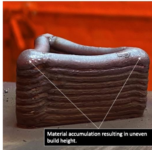
Part with uneven layer height
