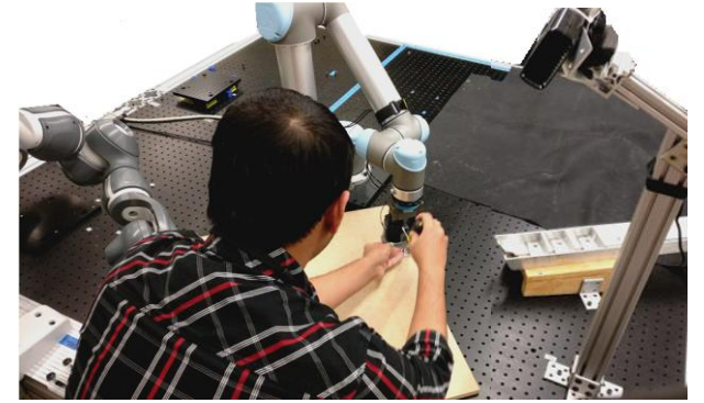
Human-robot collaborative cell for fixtureless assemblies
