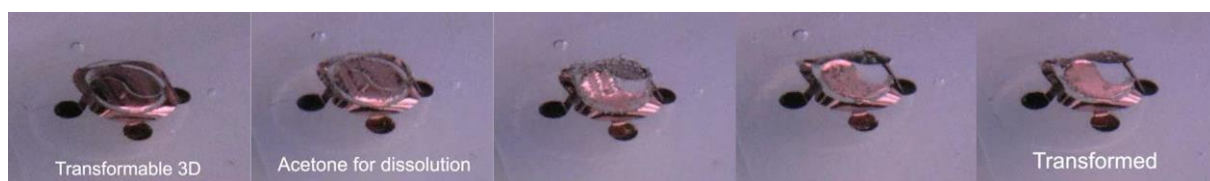
Figure S11. Captured images during transformation of 3D device from a video (transform.mp4). For accelerating dissolution of PLGA, we immersed 4D structure into a solution (Aceton:DI, 1:1) instead of PBS.
