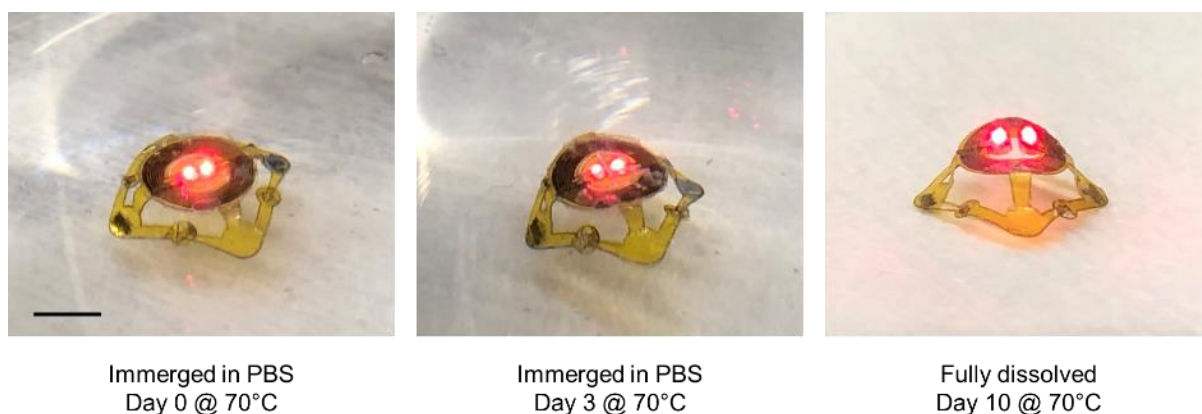
Figure S9. Photograph images of 3D electronics at various states of immersion in phosphate-buffered saline (PBS) at 70°C. Scale bar 3 mm.
