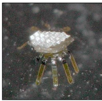
Fig. S34. Optical image of the retroreflector integrated on a robot. Scale bar, 500 \mu\text{m} .
